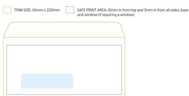
> Standard window is 28mm x 95mm, 32mm fom the left and 16mm from the base
